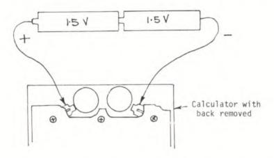
Some multitesters supply three volts to the probes for resistance measurement. Such an instrument is a convenient temporary power supply. Ensure that its batteries are in order. You can make certain of the polarity by touch-testing the resistance of a small battery in both directions.
