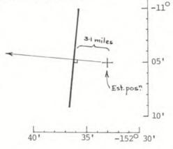
To plot the above, mark the estimated position on your chart. Place a protractor on the point and mark the azimuth. From the estimated position measure off 3.1 miles <u>towards</u> the sun and draw the position line at right angles to the azimuth. You are somewhere on this line.
